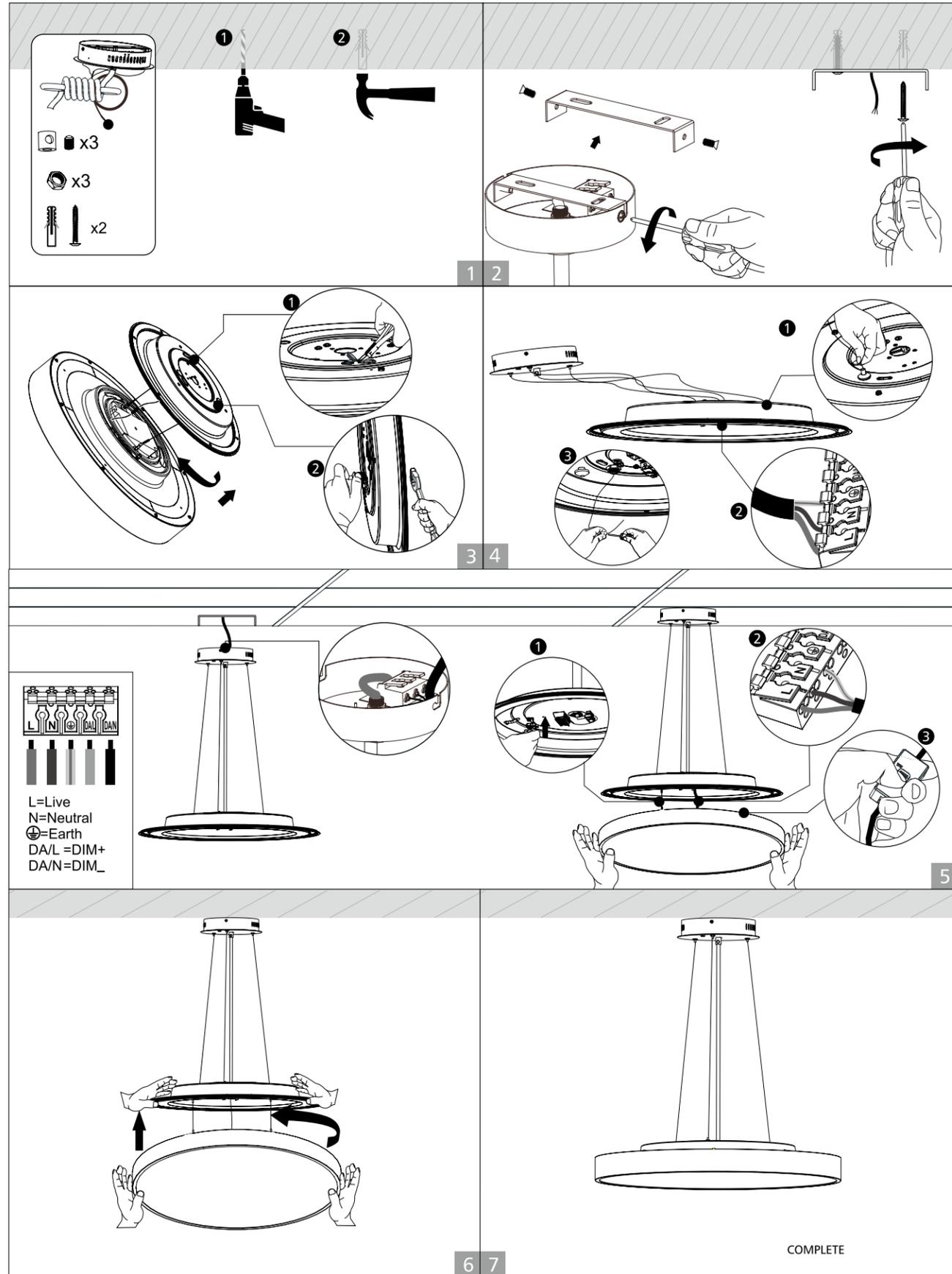
With wire harness suspension installation
