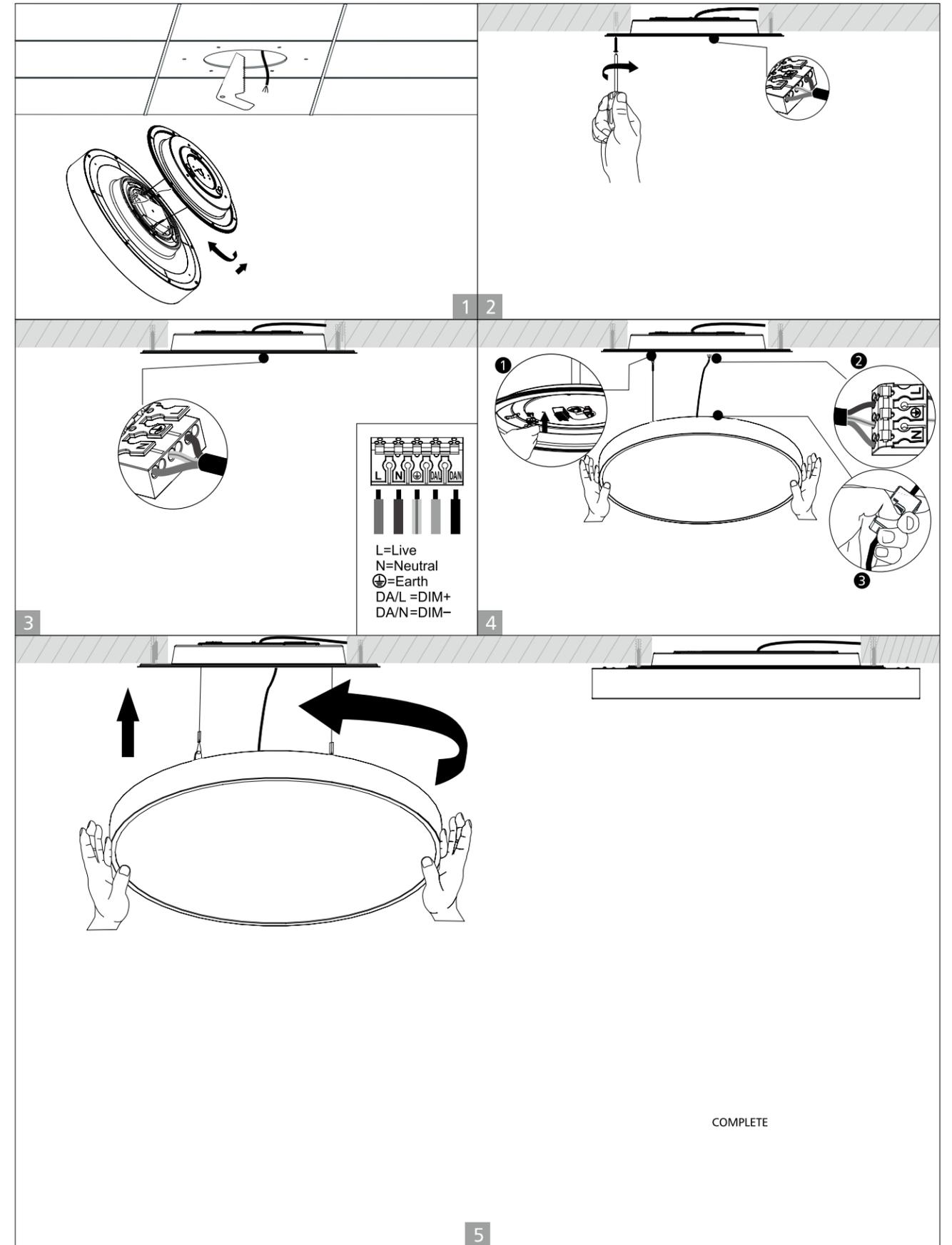
With steel wire suspension installation
